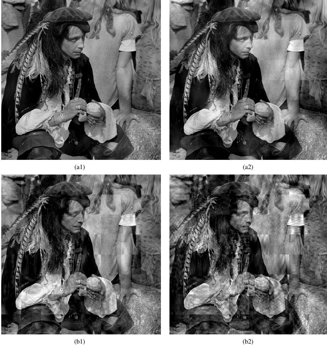
Fig. 5. (a1) shows an image transferred once with our scheme. (a2) shows the same image transferred 3 times with our scheme. In (b1) we set the \alpha -factor used by the Cox algorithm to 0.5 in order to obtain stronger watermarks for the small parts. As a result differences between adjacent document parts are visible. (b2) shows the result after 3 transfers with the stronger watermark in (b1).
